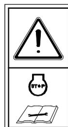
Shut off engine before performing maintenance or repair work.
