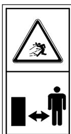
Do not stand in the machine's work area. Make sure there are no stones, twigs and other rubbish on the lawn. This type of object can be thrown by the machine and cause personal injury or damage to the machine. Avoid driving over gravel paths, etc.
