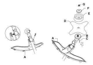
Hook the blade guard/combination guard (A) onto the fitting on the shaft and secure with the bolt.
